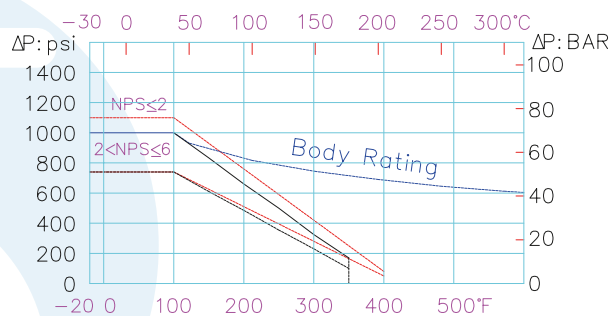
PTFE/R.PTFE Ball SEAT Pressure-Temperature RATING
